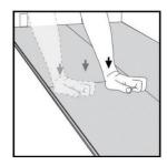
10. Last row. Minimum width 5cm. Remember to leave a 5mm expansion gap. Cut the planks lengthwise, if necessary.
